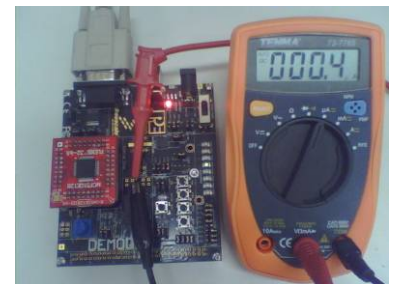
Stop 2 Measured Current: 0.4uA
